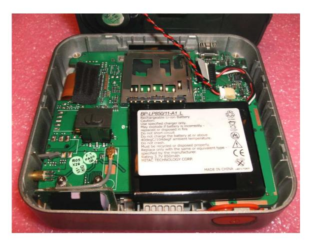
Note which corner of the battery the main board connector is closest to. When you install the replacement battery, you will want to orient the battery so that the corner which the connector cable comes from takes the shortest path to the main board connector. Leaving enough slack will ensure that things are not pulled too tight. Note that this may require orienting the replacement battery label "upside down."
