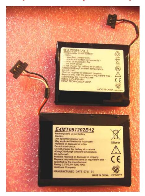
The Mio OEM C-220 Battery compared with a smaller OEM C-230 battery
